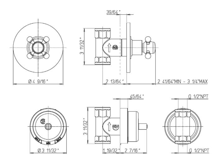
Firenze volume control 3/4" ceramic disk valve 1/2" inlet connections
