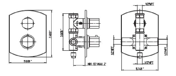
Novello thermostatic valve with 3/4" ceramic disk volume control 1/2" inlet connections
