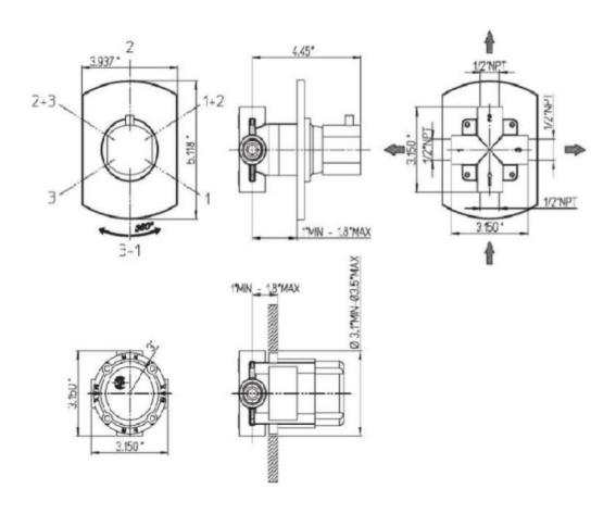
Novello 3-way diverter 3/4" ceramic disk valve 1/2" inlet connections
