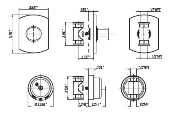
Novello volume control 3/4" ceramic disk valve 1/2" inlet connections
