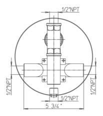
Elix thermostatic valve with ¾" ceramic disk volume control ½" inlet connetions
