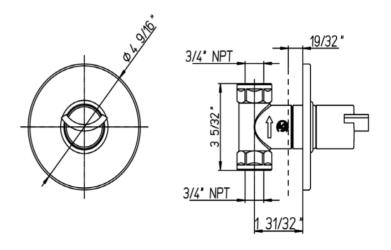
Morgana ¾" thermostatic valve only ¾" inlet connections
