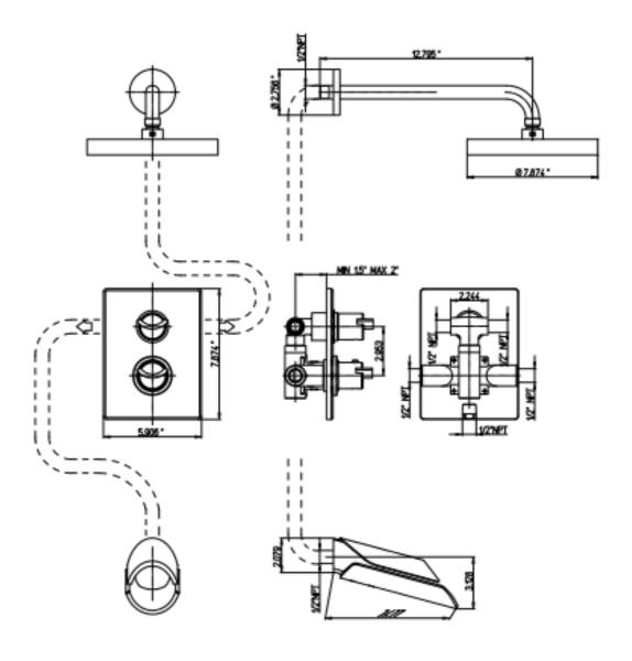
Morgana thermostatic valve with 2-way diverter volume control ½" inlet connections
