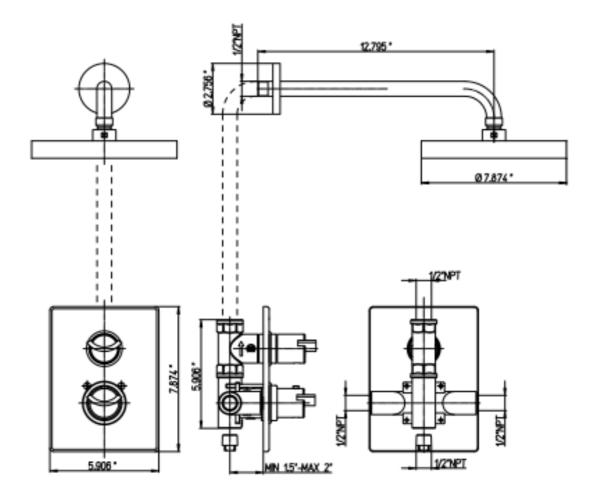
Morgana thermostatic valve with ¾" ceramic disk volume control ½" inlet connections
