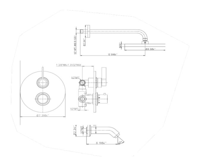
Elix thermostatic valve with 2-way diverter volume control 8"rain shower head with 12" arm Rough Included.
