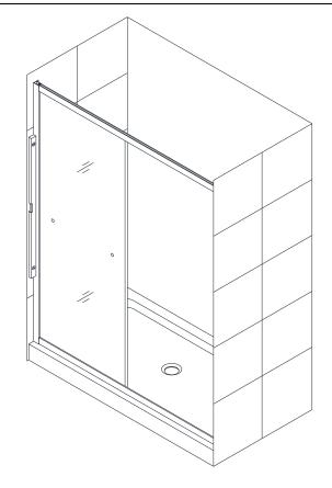
10. Using help to hold this assembly in the right position, mark the drill holes on the wall through the holes on the flange of the **Wall Profile**.
