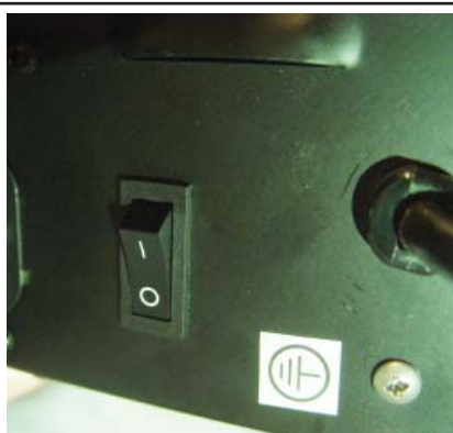
Main Power Switch in "OFF" Position.
