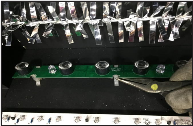
Figure 8 Light LED Replacement
