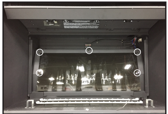
Figure 5 Flame Screen Replacement
