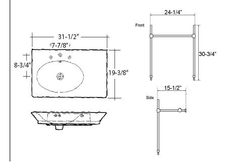
Dimensions of fixture are nominal and may vary within the range of tolerances established by ASME Standard A112.19.2. Dimensions and specifications subject to change without notice.
