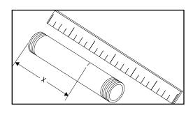
Subtract 7/18" from this measurement. This is the length of the brass nipple needed.
