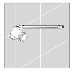
Remove the test nipple.
