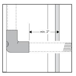
When the finished wall is complete, mark the test nipple at the surface of the finished wall.
