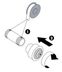
Screw the bodyspray/nipple assembly into the ell. Tighten the bodyspray using a wrench.
