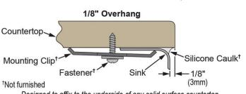
Designed to affix to the underside of any solid surface countertop.
