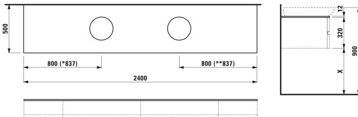
\* = Only II Bagno Alessi One 81897.3 with shelf at left side / \*\* = Only II Bagno Alessi One 81897.3 with shelf at right side X = The exact hight must be set during installation.
