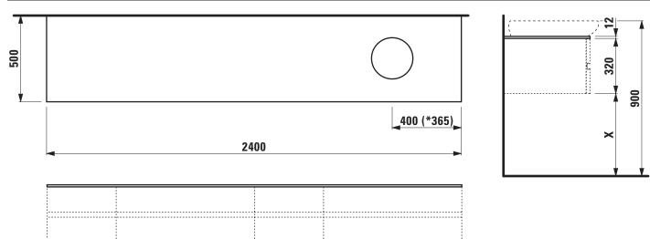
$^{\star}$  = Only II Bagno Alessi One <code>\$1897.3</code> with shelf at left side X = The exact hight must be set during installation.
