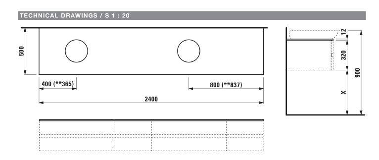
$<sup>^{\</sup>star\star}$  = Only II Bagno Alessi One  $\approx \! 1897.3$  with shelf at right side X = The exact hight must be set during installation.
