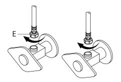
Attach waterlines (E) to angle stops and tighten until snug. Turn on angle stops and check for leaks (DO NOT TURN FAUCET ON).
