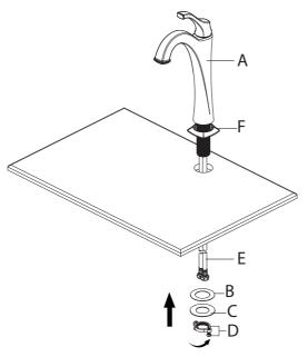
Before installation, ensure that the flange (F) is placed on the bottom of the faucet assembly (A). Place the faucet (A) through the hole in the countertop. Secure the faucet (A) to the countertop using the plastic washer (B), metal washer (C) and nut & screws (D) provided. Hand tighten the nut onto the end valve shank. Lock the nut into position by tightening the screws (D) with a phillips screwdriver.
