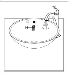
After installing the faucet, remove the aerator (G) with the included aerator key (H). Turn the water on for 30 seconds to remove any debris. Reassemble the aerator (G).
