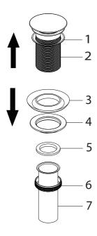
Unscrew the nut (6) from the pop-up body (2), move over the tail pipe (7) and washer (5), then unscrew the coupling nut (4) and remove the washer (3).
