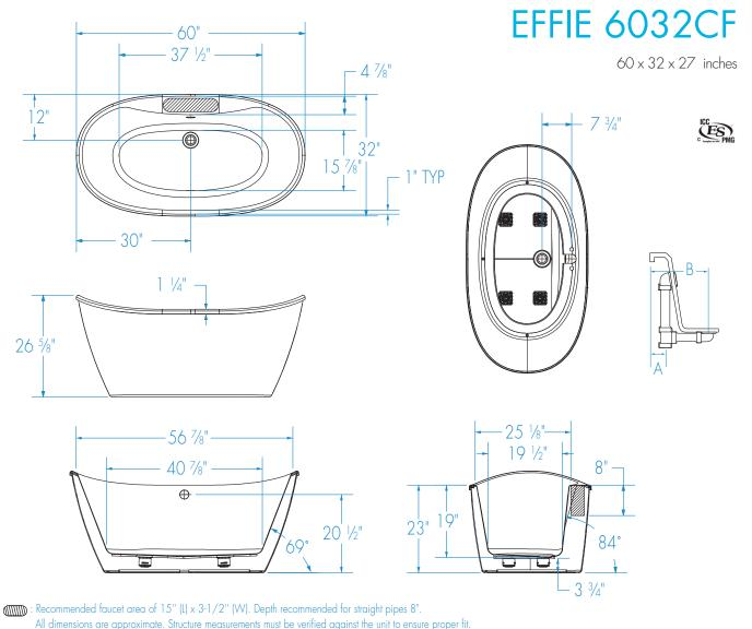
$\label{eq:FEATURES} \textbf{ Dimensional Tolerance} \pm 3/8\text{''}. \textbf{ Dimensions needed for site preparation should be measured from the unit. Manufacturer assumes no responsibility for preparatory work.}$
