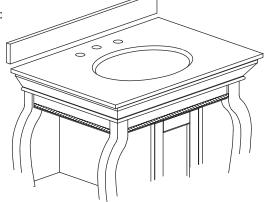
Finally, place the bottom side of back splash with sealant onto the countertop and check alignment of backsplash. Adjust the leg levelers as needed
