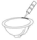
Apply continuous bead of quality sealant evenly to the top of sink flange
