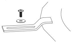
Check alignment of sink again and tighten fasteners to secure sink
