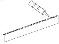
Apply silicone sealant evenly along the bottom of backsplash and wall
