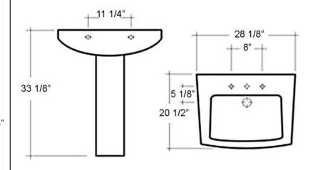
Dimensions of fixture are nominal and may vary within the range of tolerances established by ASMEI Standard A112.19.2-2013. Dimensions and specifications subject to change without notice.
