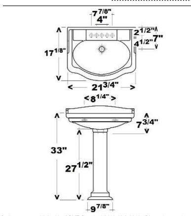
Dimensions of fixture are nominal and may vary within the range of tolerances established by ASME Standard A112.19.2-2013. Dimensions and specifications subject to change without notice.
