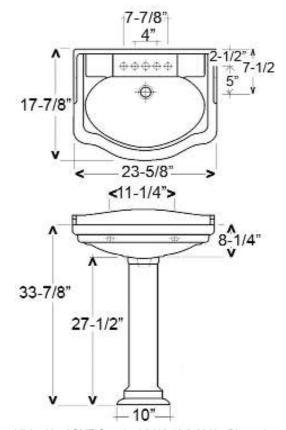
Dimensions of fixture are nominal and may vary within the range of tolerances established by ASME Standard A112.19.2-2013. Dimensions and specifications subject to change without notice.
