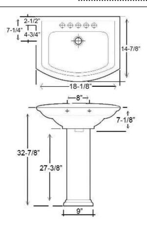
Dimensions of fixture are nominal and may vary within the range of tolerances established by ASMEI Standard A112.19.2-2013. Dimensions and specifications subject to change without notice.
