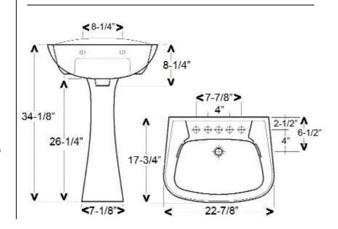
Dimensions of fixture are nominal and may vary within the range of tolerances established by ASME Standard A112.19.2-2013. Dimensions and specifications subject to change without notice.
