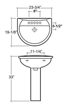
Dimensions of fixture are nominal and may vary within the range of tolerances established by ASME Standard A112.19.2-2013. Dimensions and specifications subject to change without notice.
