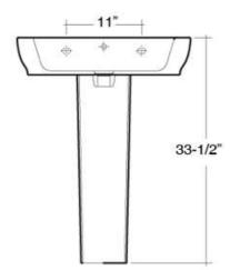
Dimensions of fixture are nominal and may vary within the range of tolerances established by ASME Standard A112.19.2-2008. Dimensions and specifications subject to change without notice.
