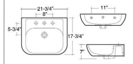
Dimensions of fixture are nominal and may vary within the range of tolerances established by ANSI Standard A112.19.2. Dimensions and specifications subject to change without notice.
