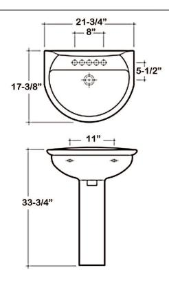
Dimensions of fixture are nominal and may vary within the range of tolerances established by ASME Standard A112.19.2-2008. Dimensions and specifications subject to change without notice.
