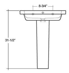
Dimensions of fixture are nominal and may vary within the range of tolerances established by ASME Standard A112.19.2-2013. Dimensions and specifications subject to change without notice.
