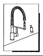
5. After installing faucet, remove spray assembly and open the hot and cold water supplies. Check for leaks. Turn on faucet handle for one minute to flush debris from faucet. Close the handles and re-assemble the spray.
