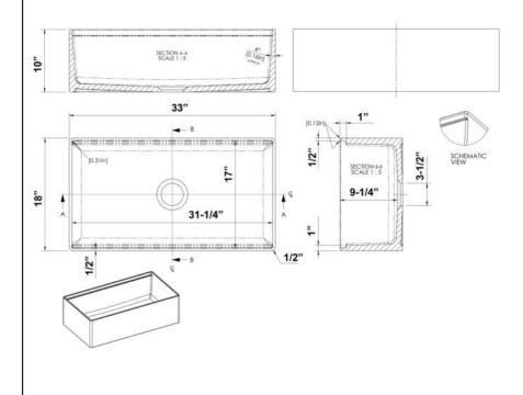
Dimensions of fixture are nominal and may vary within the range of tolerances established by ANSI Standard A112.19.2.2018 Dimensions and specifications subject to change without notice.
