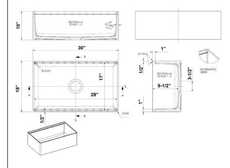
Dimensions of fixture are nominal and may vary within the range of tolerances established by ANSI Standard A112.19.2.2013 Dimensions and specifications subject to change without notice.
