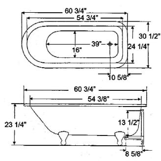
Dimensions of fixture are nominal and may vary within the range of tolerances established by ANSI Standard A112.19.2. Dimensions and specifications subject to change without notice.
