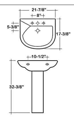
Dimensions of fixture are nominal and may vary within the range of tolerances established by ASME Standard A112.19.2-2008. Dimensions and specifications subject to change without notice.
