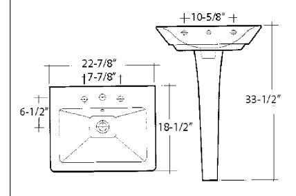
Dimensions of fixture are nominal and may vary within the range of tolerances established by ASME Standard A112.19.2. Dimensions and specifications subject to change without notice.
