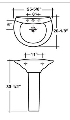
Dimensions of fixture are nominal and may vary within the range of tolerances established by ASME Standard A112.19.2-2008. Dimensions and specifications subject to change without notice.
