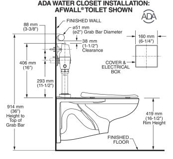
\*\* Flush Valve can be installed to meet ADA 2010 Section 609 when installed as shown
