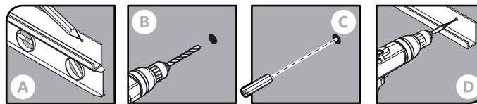
Drill the holes in the wall with a 3/16" drill bit.
