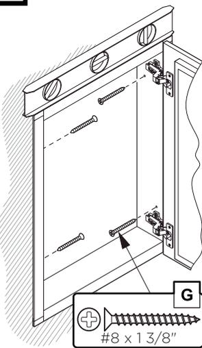
Level, then secure the medicine cabinet with the screws (**G**) through the mounting holes into the framing studs.
