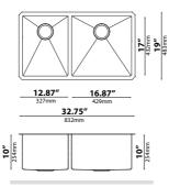
KHU104-33 32 3/4" x 19" x 10" Min Cabinet Size: 36" Matching Grid: KBG-104-33-1 and KBG-104-33-2 Drain Model #: BST-1 & ST-1
