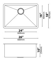
KHU100-26 26" x 18" x 10" Min Cabinet Size: 30" Matching Grid: KBG-100-26 Drain Model #: ST-1
