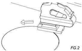
2. Cut out the counter -The cutting tools required will depend on the surface to be cut. FG.2 (Your sink comes with 4 mounting screws for mechanical fastening. Screws are only nesecary if for some reason silicone cannot be used. In this case, you will need to drill 4 holes in the counter to accommodate these screws)
