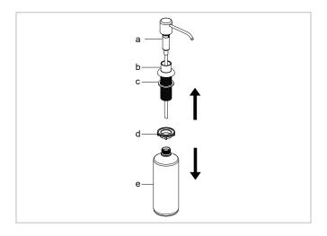
Install dispenser base (b) with washer (c) attached into the hole in the countertop. Re-install mounting nut (d) on the dispenser base (b) from underneath the countertop. Tighten mounting nut (d) by hand
