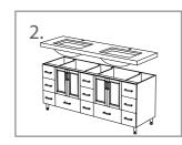
1.Apply continuous stream of quality silicon glue on top of the cabinet contact area.
