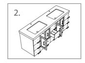
1. Hold the handles, unscrew the screws from doors and drawers. 2.Put the screws inside and handles outside gently, tighten the
