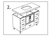
1.Apply continuous stream of quality silicon glue on top of the cabinet contact area.2.Place the counter top on top of the cabinet.
