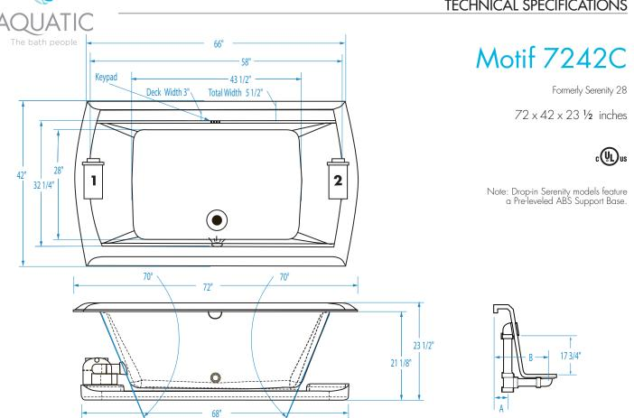
**FEATURES** Dimensional Tolerance ± 378". Dimensions needed for site preparation should be measured from the unit. Manufacturer assumes no responsibility for preparatory work.
