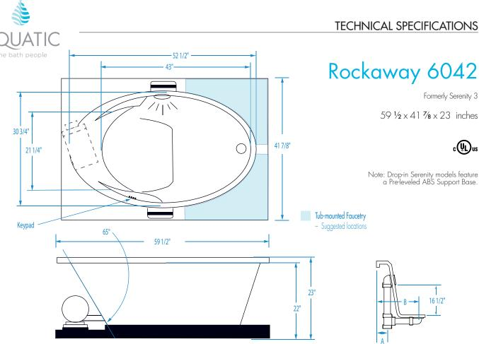
**FEATURES** Dimensional Tolerance ± 3/8". Dimensions needed for site preparation should be measured from the unit. Manufacturer assumes no responsibility for preparatory work.
