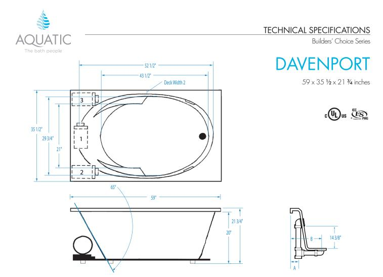
FEATURES Dimensional Tolerance ± 3/8". Dimensions needed for site preparation should be measured from the unit. Aquatic assumes no responsibility for preparatory work.
