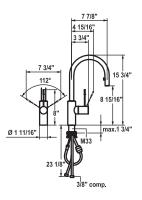
KWC-No. Finish 10.151.102.000 chrome A 7 1/8", flexible connection hoses solid stainless steel 10.151.102.700 A 7  $\frac{7}{8}$ ", flexible connection hoses 10.151.102.000DL chrome A 7 % " , flexible connection hoses 10.151.102.700DL solid stainless steel
