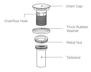
**STEP 3:** From under the drain, insert the think rubber washer and screw on and tighten the metal nut. Remove excess plumbers' putty. See Figure 3.
