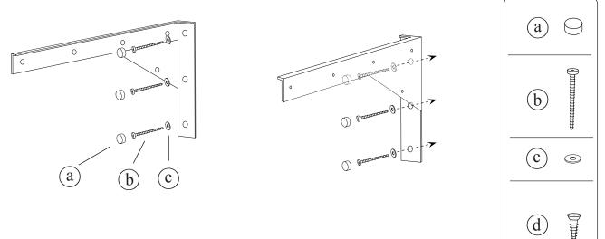
Step 2 : Attach the cabinet to the wall bracket.
