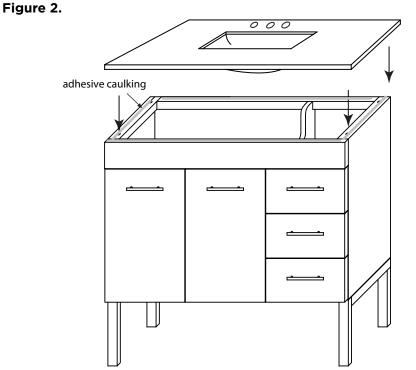
**STEP 3:** Apply adhesive on wood bracket and mounting surfaces of the cabinet *See Figure 2.*
